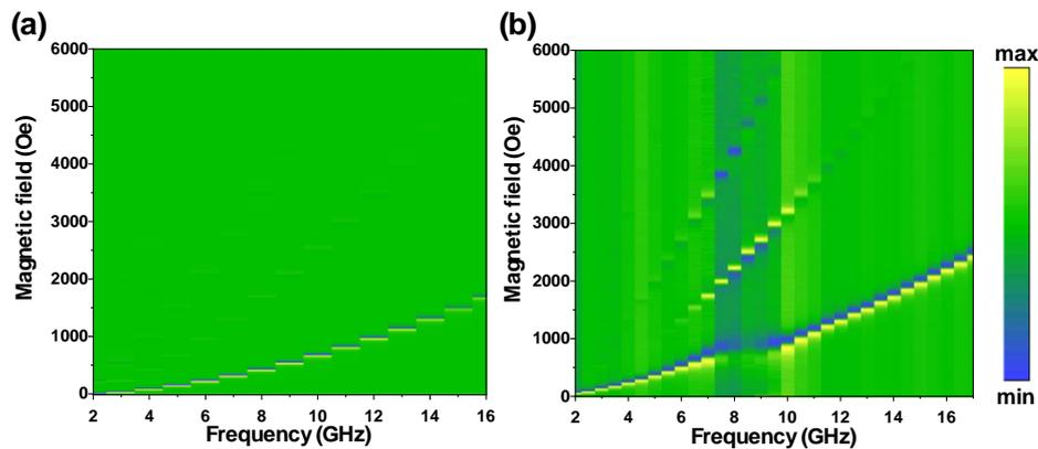
Fig. 1. FMR signal on sweeping magnetic field and microwave frequency in two different SAFs: (a) CoFeB(10)/Ru(0.42)/CoFeB(5) and (b) CoFeB(5)/Ru(1)/CoFeB(2.5). The numbers in parentheses are the layer thicknesses in nanometres (nm). The colour bar on the right side corresponds to the FMR signal.
